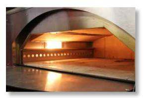
The arched refractory brick-lined ceiling of the MB Series ovens develop more heat synchronization, enabling the oven to maintain temperature more efficiently and evenly.
